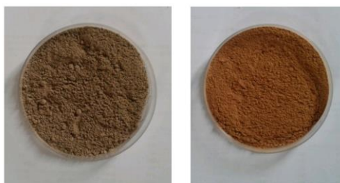
Figure 3: Physical appearances of a) raw corn stover ash (RCSA) b) corn stover digestate ash (CSDA).
