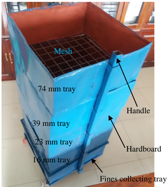
Figure 6: Arrangement of mesh during measurement of hand crushed rocks.
