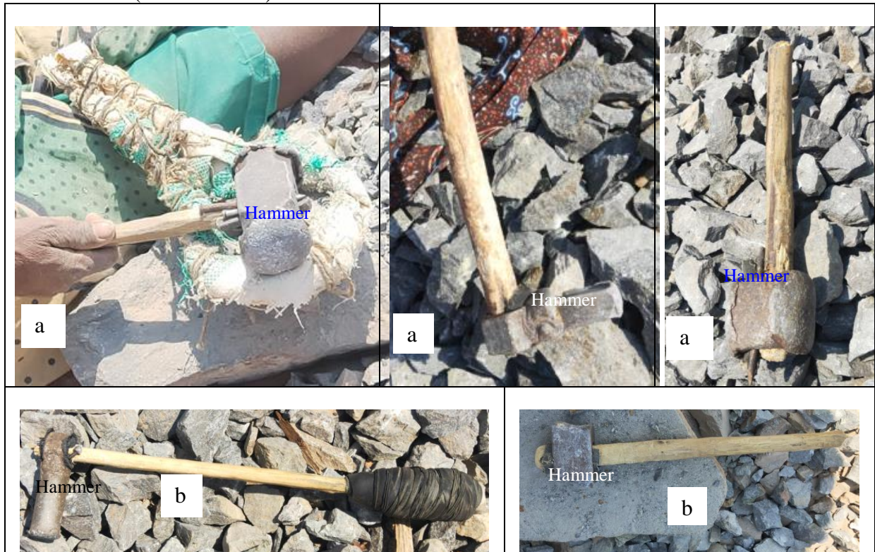
Figure 1: Different types of hand-hammers with wood handles for crushing rocks (a) with two sides for crushing rocks (b) One side for crushing rocks.
