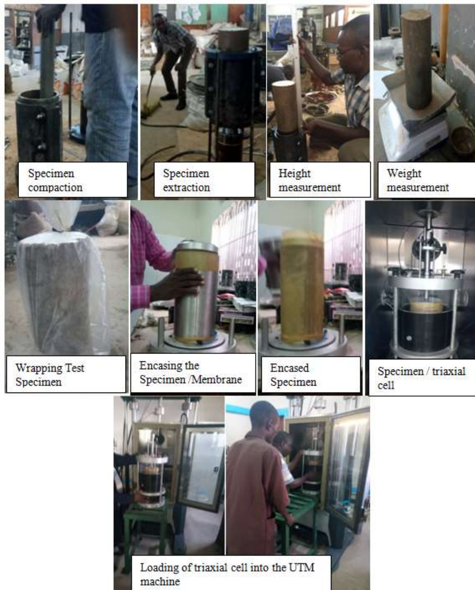
Figure 7: Preparation of specimen for M_r testing
