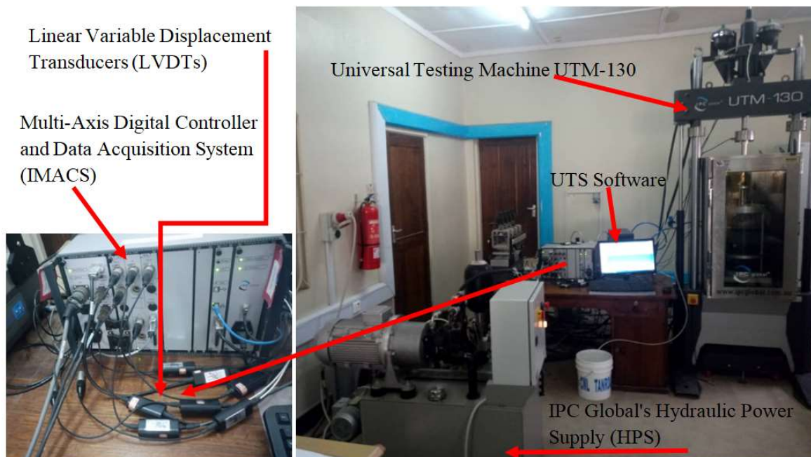
Figure 6: Universal Testing Machine UTM-130 set-up for M_r testing
