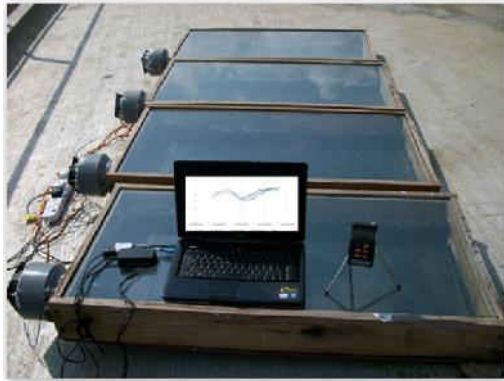
Figure 11: General experimental setup of flat plate solar collector
