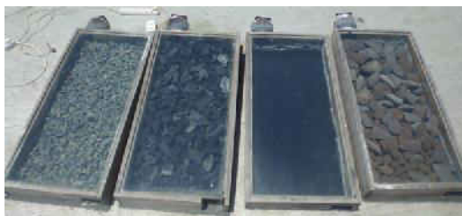
Figure 14: Solar collector, from left, with granite gravels, charcoal, galvanized steel plate and porous rocks
