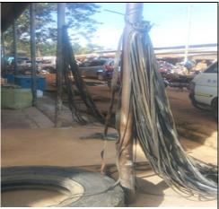
Elastic straps made out of vehicle tubes
